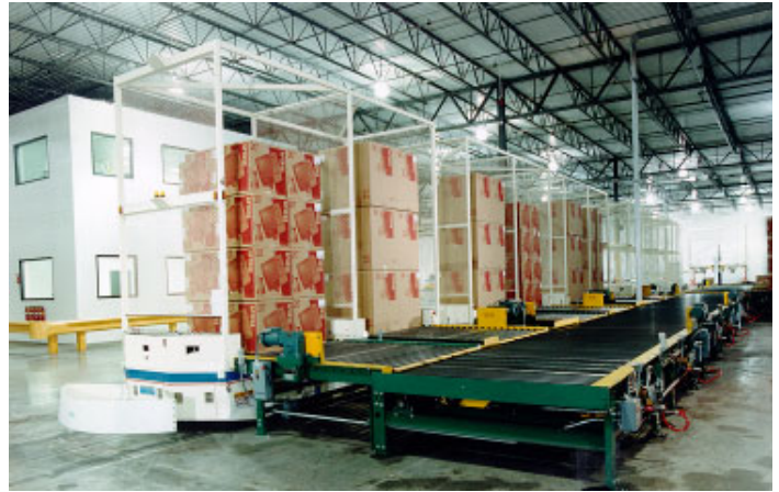
Two AGVs parked at the unitizer output "C" waiting load pick-up via right angle transfer.
