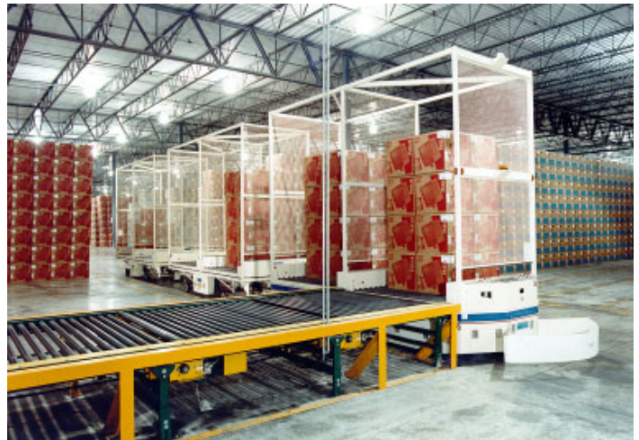
AGV at a typical drop off station carrying six loads per train.
