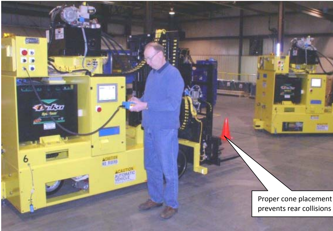
Figure 2: The traffic cone placed to the rear of the AGV under pendent control reduces the possibility of a collision by the approaching AGV.
