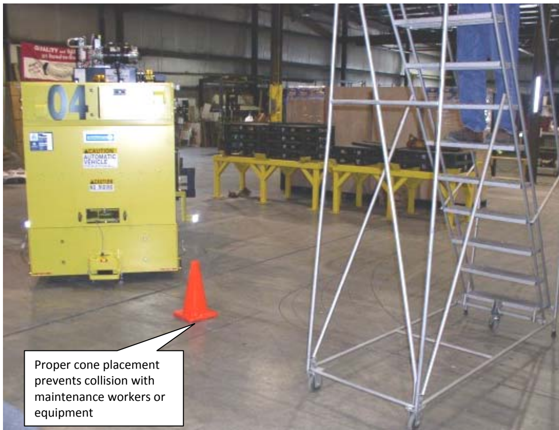
Figure 3: Illustrating proper traffic cone placement.
