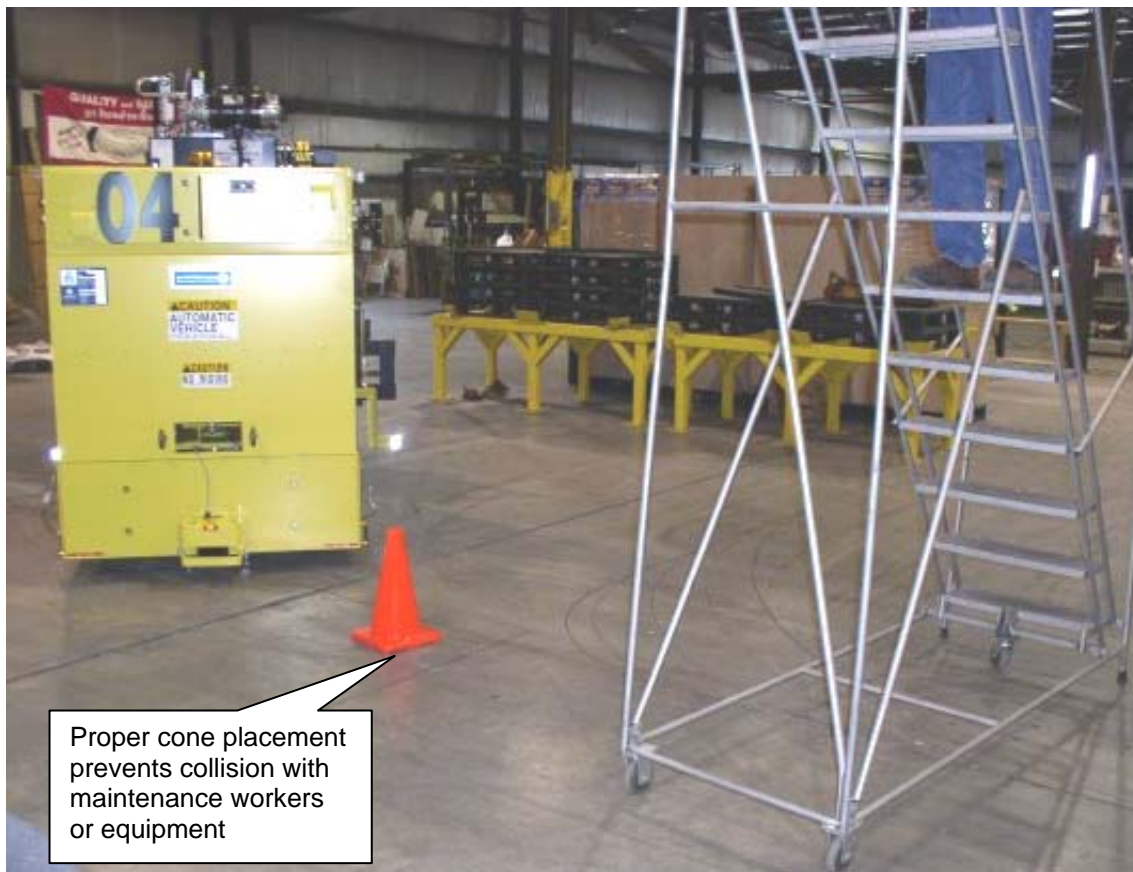
Figure 3: Illustrating proper traffic cone placement.
