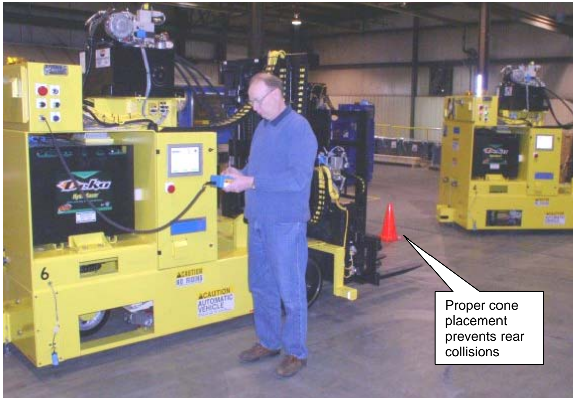
Figure 2: The traffic cone placed to the rear of the AGV under pendant control reduces the possibility of a collision by the approaching AGV.
